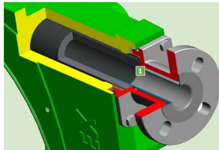
1 When fitted with hygienic flanges (e.g. DIN 11851, Triclamp or RJT) the pump meets EHEDG Standards
